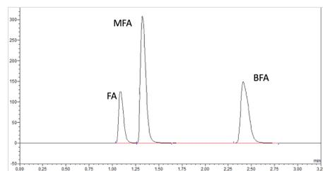
Figure 7. Chromatogram of a typical esterification reaction. Hydrolysis product FA, substrate MFA and desired product BFA appear as single peaks.
