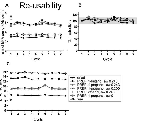
Figure 10. Re-usability of immobilised B1. A) Product formation per hour per g FAE. B1 enzyme was immobilised on SBA-15 10.2 nm and either dried conventionally, or rinsed with a solvent. Reaction was run over 9 reaction cycles. B) Loss of activity over 9 consecutive reaction cycles, expressed as percent of original activity. C) Loss of activity over 9 consecutive reaction cycles, expressed as percent of original activity.
