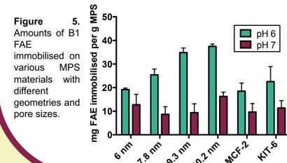
Figure 5. Amounts of B1 FAE immobilised on various MPS materials with different geometries and pore sizes.
