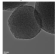
Figure 2. TEM image of SBA-15 mesoporous silica. Image credit: wikipedia
